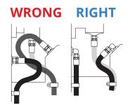
Obtain direct routing of hose through use of 45° and 90° adapters and fittings. Improve appearance by avoiding excessive hose length.
