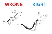
Adequate hose length is most important to distribute movement on flexing applications and to avoid abrasion
