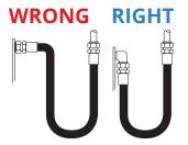
Avoid sharp twist or bend in hose by using proper angle adapters.
